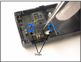
Note: The snaps on either side must clear the retainers.
