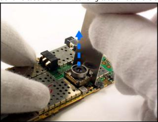
B. Use opposite end of tool to lift camera from its mount. Be careful not to damage any contacts.
