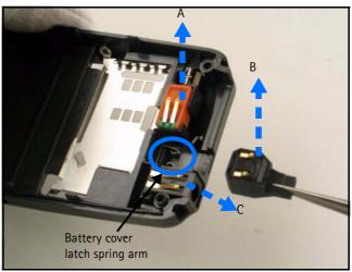
Note: Be aware of the battery cover latch spring arm. It might fall out, due to its placement underneath the microphone assembly.
