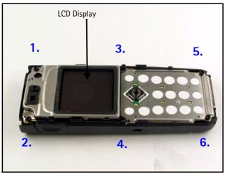
B. Place protective film on the LCD display to prevent scratches.
