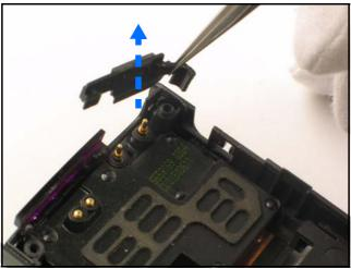
Note: The other end of the power key will separate from the IR lens.
